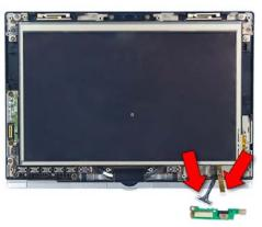
9. Connect the 2 cables to the new power switch board and place it into the rear cover.
