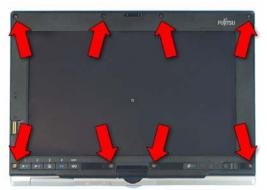
11. Press the front cover into place and secure it with 8 screws.
